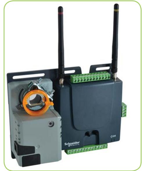
The device has a pressure sensor and is equipped with an optional damper actuator. The device also has optional embedded EnOcean and ZigBee wireless modules to enable bidirectional communication with EnOcean and ZigBee devices. The Managers can communicate with each other wirelessly using their ZigBee modules.
